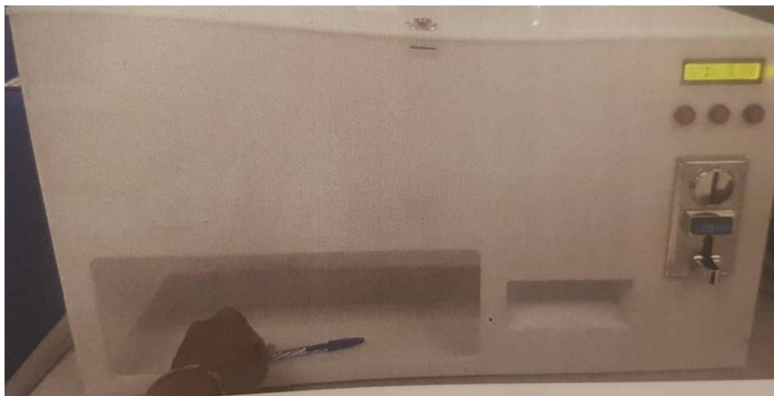
Fig. 3 The output prototype of the pen vending machine
